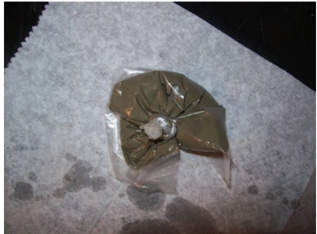
Figure 3.14 Folded plastic bag with a knot, to be placed inside the sample holder.
