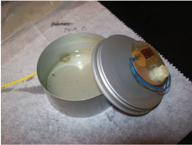
Figure 3.10 Sample holder filled with oil and the lid on which the heater is mounted.
