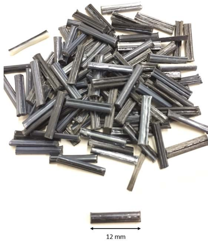
Figure 3.2.: Long discontinuous carbon fiber-reinforced PPS pellets produced using pultrusion.
