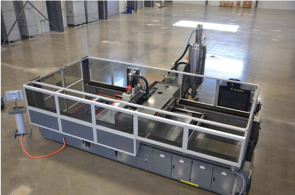
Figure 1.8.: Big Area Additive Manufacturing or BAAM system developed by Oak Ridge National Lab (ORNL) and Cincinnati Incorporated (CI) [14].
