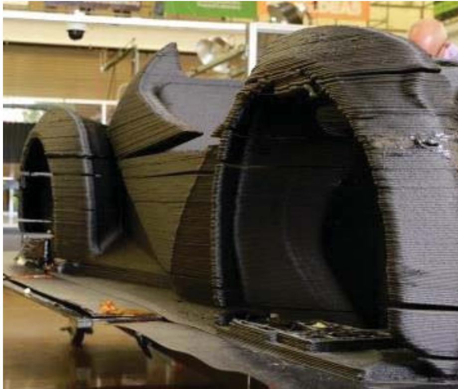
Figure 1.10.: Layer delamination that occurred in an early attempt to 3D print a car [15].
