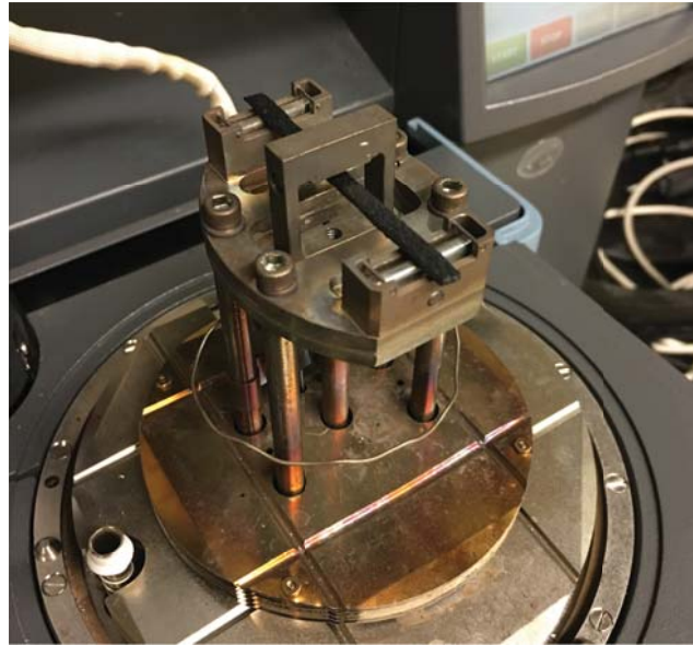
Figure 6.7.: Sample loaded in the 50 mm span 3 point bending clamp.
