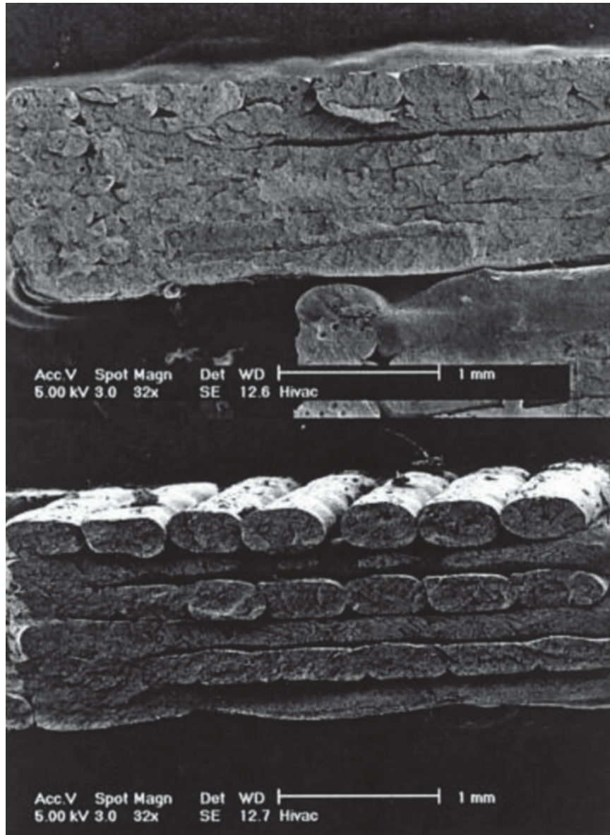
Figure 1.5.: SEM images of fracture surfaces of 10^\circ/90^\circ FDM samples from neat ABS (top) and VGCF/ABS composite (bottom) [5].
