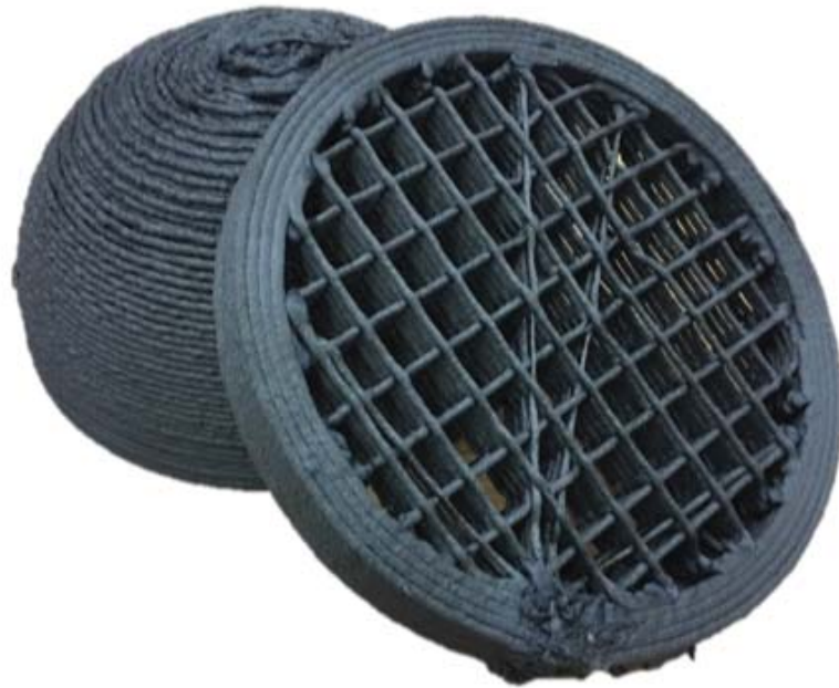
Figure 4.3.: Parts printed from 50 weight percent carbon fiber-reinforced PPS on an AM machine developed at Purdue University.
