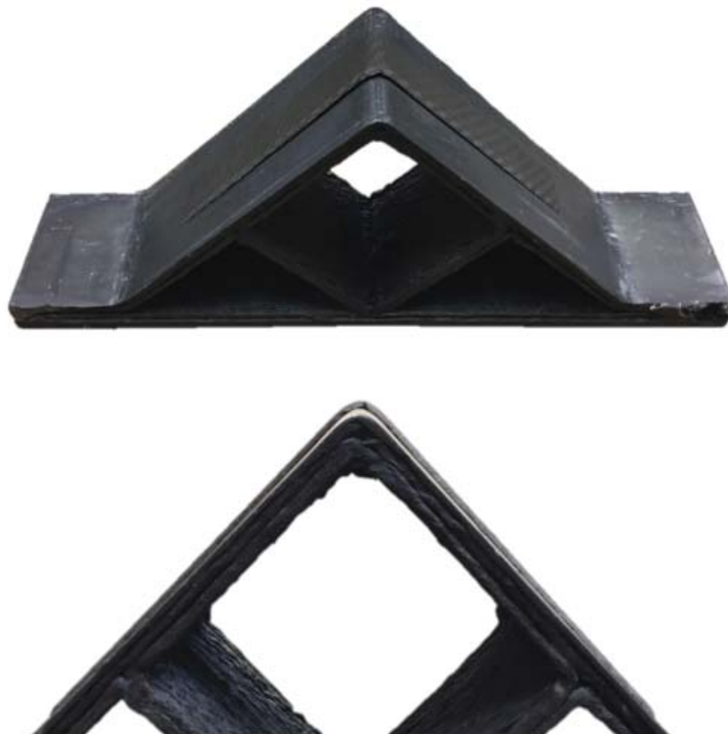
Figure 4.5.: top) The bracket prior to removal from the tool; bottom) Observed gap between tool and part surface.
