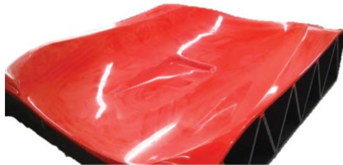
Figure 4.2.: Large composite tool printed from carbon fiber-reinforced-ABS on a BAAM machine developed by ORNL and CI.
