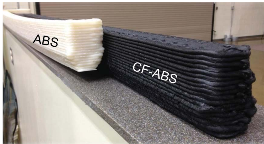
Figure 1.9.: Decreased warpage in carbon fiber-reinforced printed bar [15].
