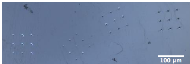
Figure 2.1. The arrays of 9 indents at different angles, the rightmost being zero degrees with increasing angle to the left.
