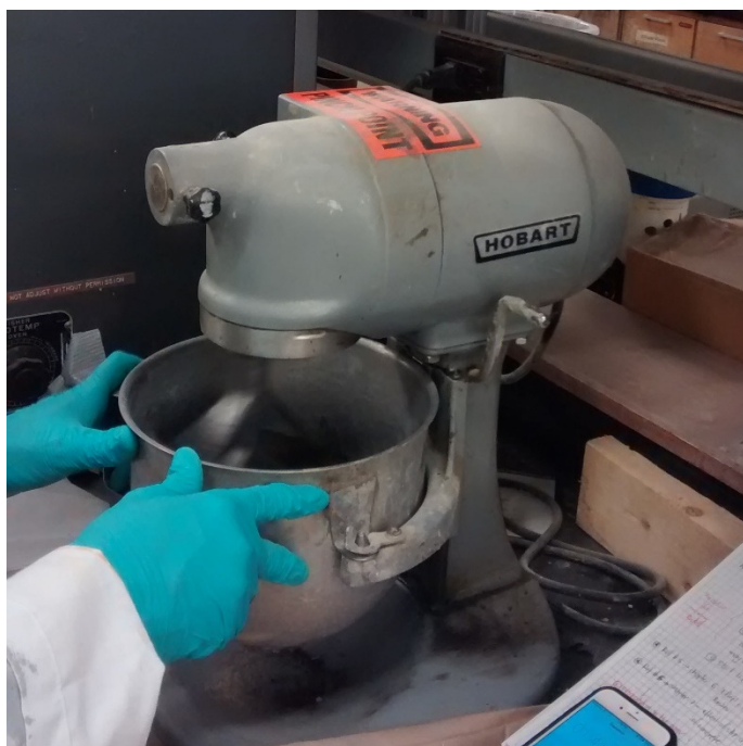
Figure 13 - Mixing of cement paste using a Hobart mixer following ASTM C305-14
