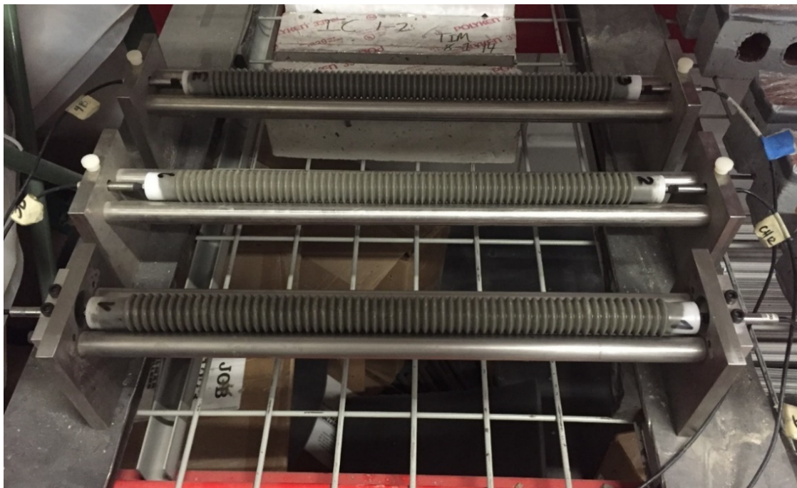
Figure 52 –Autogenous shrinkage test of cement paste - ASTM C1698 – 09 (Reapproved 2014), “Standard Test Method for Autogenous Strain of Cement Paste and Mortar”.
