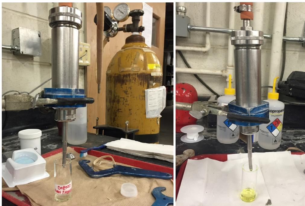
Figure 15 - Pore solution extraction from fresh cement paste by means of Millipore™ pressure filtering system.
