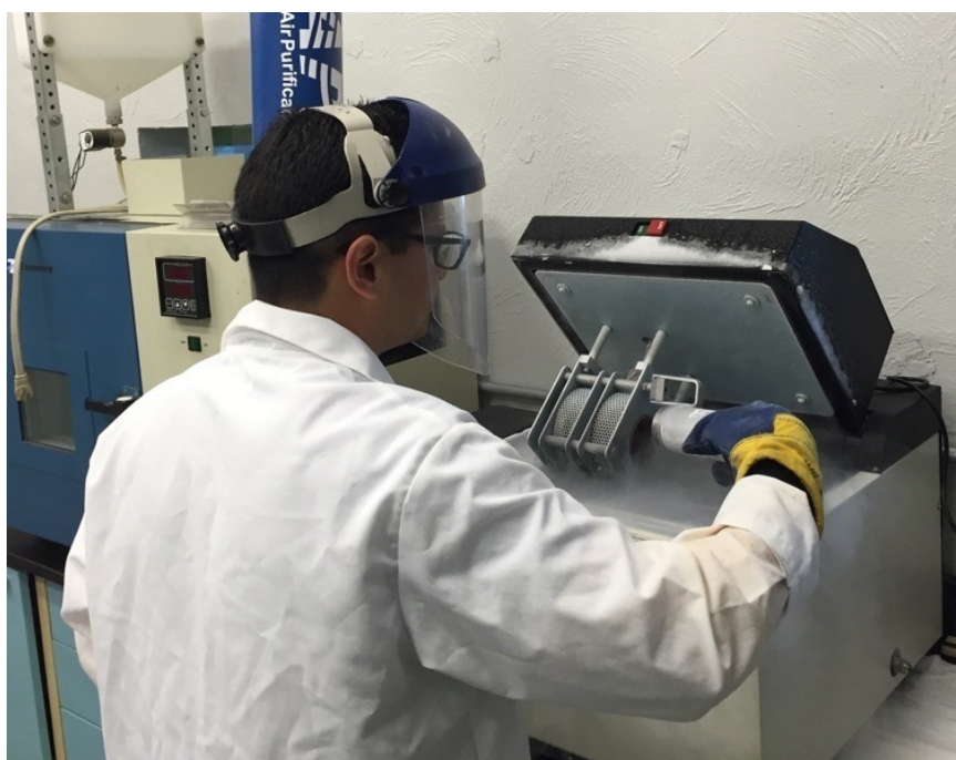
Figure 21 - Extraction of SAP sample after milling process
