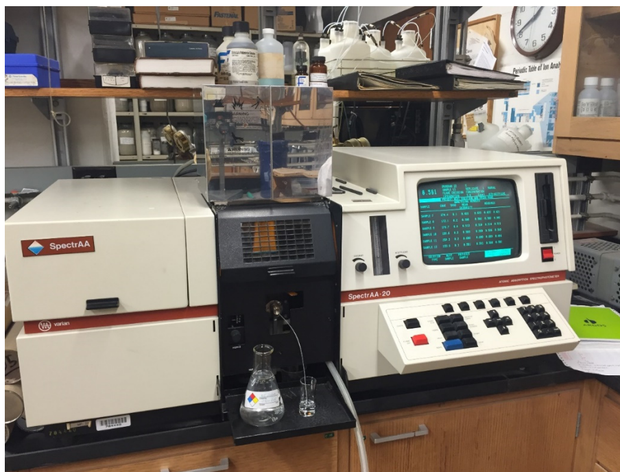
Figure 18 - Sample tested for determination of cations using VARIAN SpectrAA 10/20
