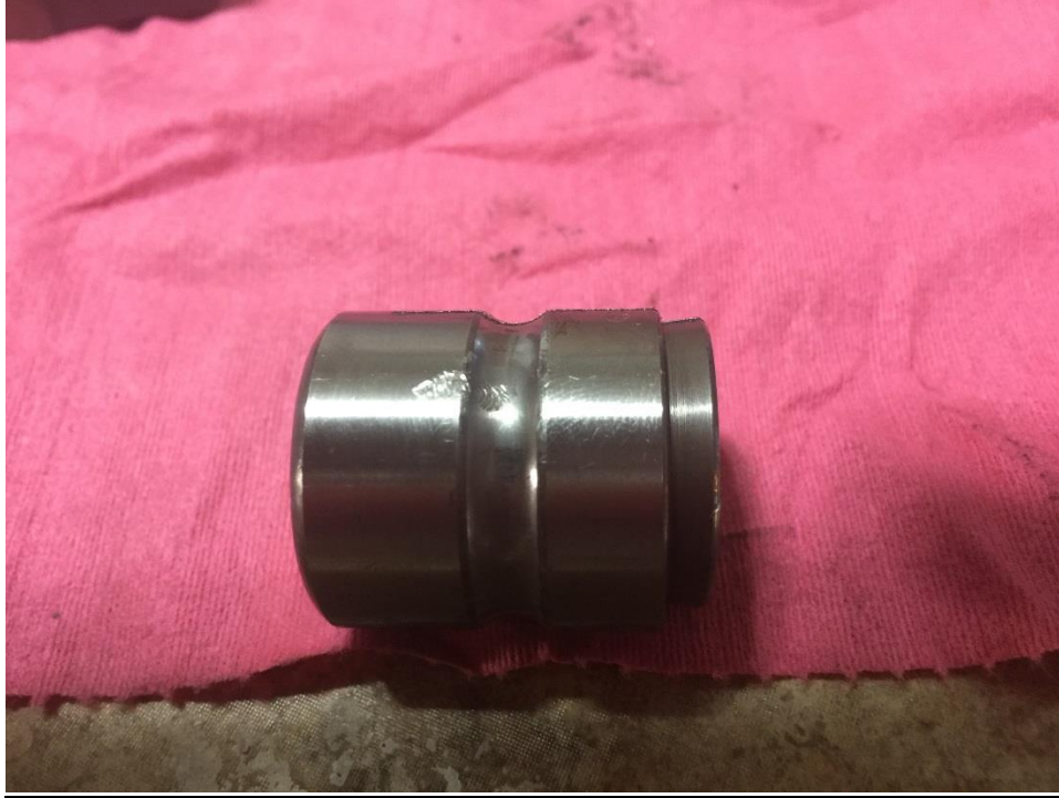
Figure 4.23 Test bearing inner race (phase 3 fault).
