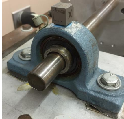
Figure 4.1. Test bearing with triaxial accelerometer mounted
