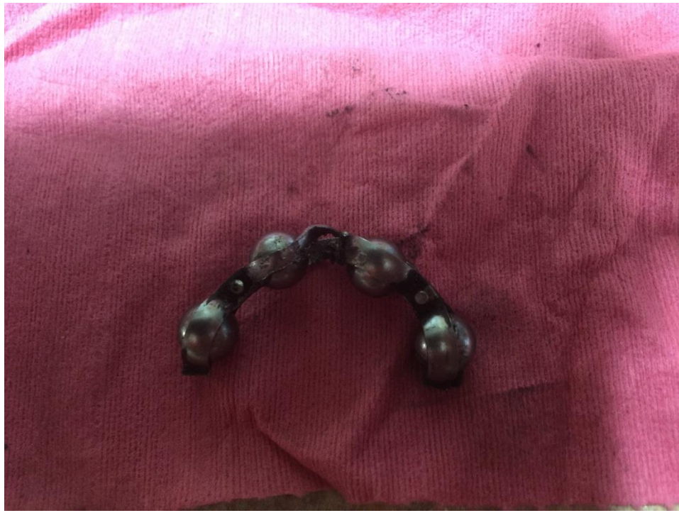
Figure 4.24. Test bearing cage damage (phase 3 fault)
