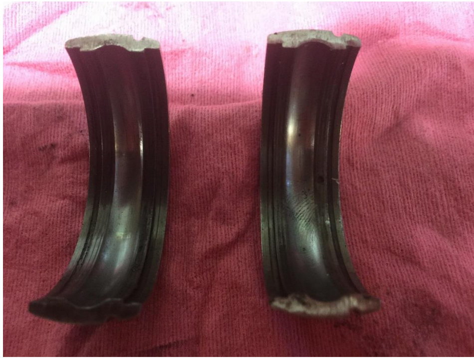
Figure 4.22 Test bearing outer race (phase 3 fault).
