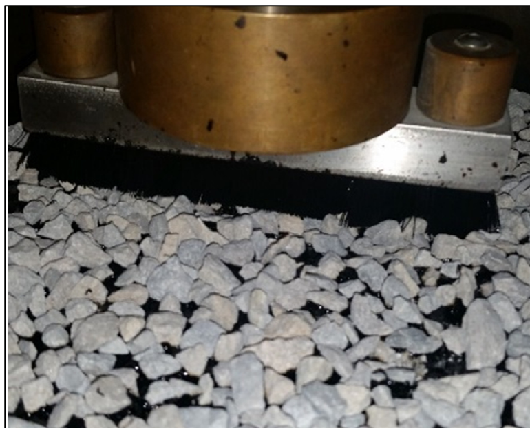
Figure 3.16: ASTM D7000 brooming simulation.
