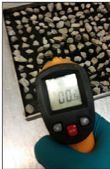
Figure 3.19: Specimen temperature after freezer conditioning, 0 \pm 2^\circ\text{C} .
