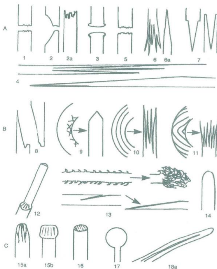
Figure 17. Different types of fractures in fibers. Group A- Tensile breaks : (1) brittle, (2) ductile, (2a) light-degraded, (3) high-speed mushroom, (4) axial splits, (5) granular, (6) fibrillar, (7) stake-and-socket. Group B-Fatigue : (8) strip and tail, (9) kink bands, (10-11) splits, (12) wear, (13) peeling, (14) rounding. Group C-Others : (15) mangled, (16) cut, (17) melted, (18) natural end of cotton fiber. This figure was taken from 54 .
