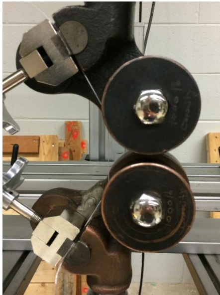
Figure 23. Fixture used for tensile testing.
