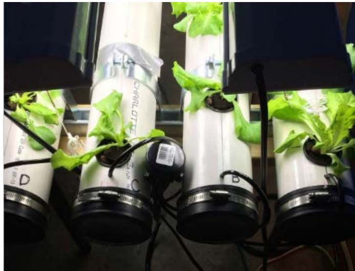
Figure 3.11. Delivery manifold with tubing delivering water to each PVC pipe.
