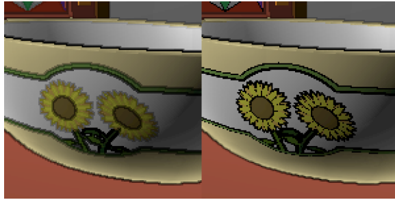
Figure A.3. These cropped portions of side-by-side NPR renders illustrate the partial-darkening effect for thin lines. On the right, the baked-lines method displays lines less than two pixels thick; the dynamic method draws thicker lines, but it dims them to compensate.
