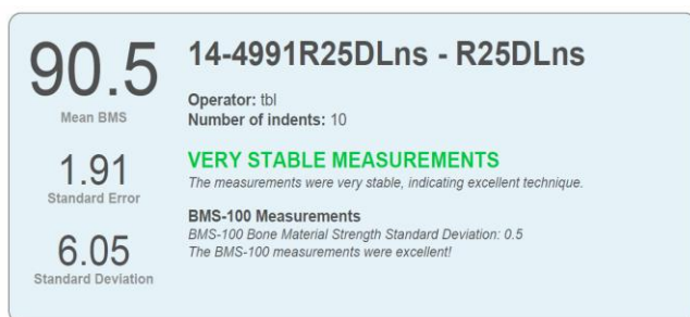
Figure 3. Typical report from the Osteoprobe. Measurements are either described as ‘Very Stable’, ‘Stable’ or ‘Unstable’, where the last case implies that the tests should be repeated.
