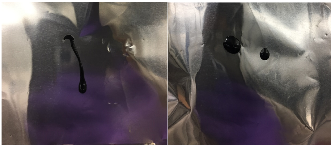
Figure 3-1. Fluid characterization for electrode mixture with different CB content (Left: 0%, Right: 5%).
