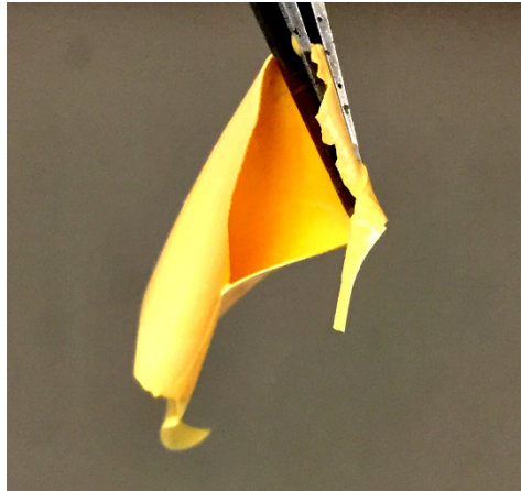
Figure 3-3. PEG mixed with \text{Al}_2\text{O}_3 nanoparticles after photo-curing.
