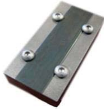
Figure 4 The Almen strip of the Almen Intensity test, fixed in position prior to being exposed to shot peening. 23
