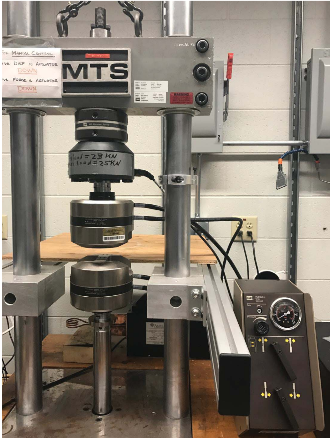
Figure 35 MTS load frame, illustrating hydraulic grips, test frame, and grip control panel.
