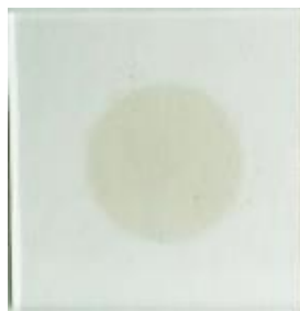
Figure 2.9. Deposited, Transparent MoS 2 Film on ITO Coated Glass Substrate.
