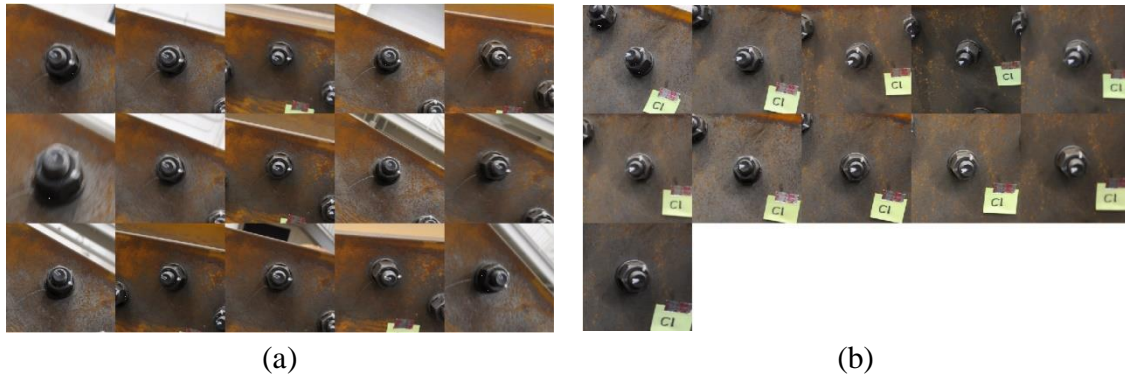
Figure 2.8 Resulting groups of object patches at crack locations A and B in Fig. 2.6.
