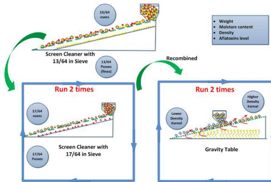
Figure 2.3 Diagram showing size and density segregation tests conducted at a commercial inbred seed processing facility.
