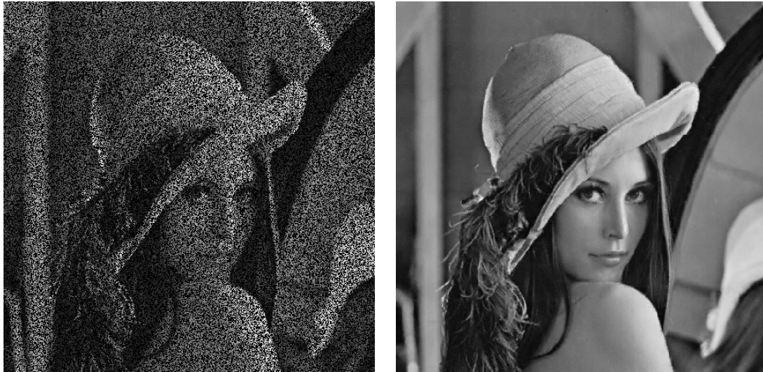
Figure 4.14. Image Inpainting. Left: lena with 50% of the data removed. Right: Inpainting result from global learned dictionary using GSCAD.
