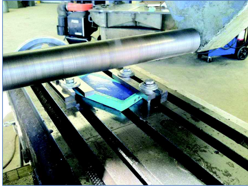
Figure 5.7: Milling machine scribing a steel plate
