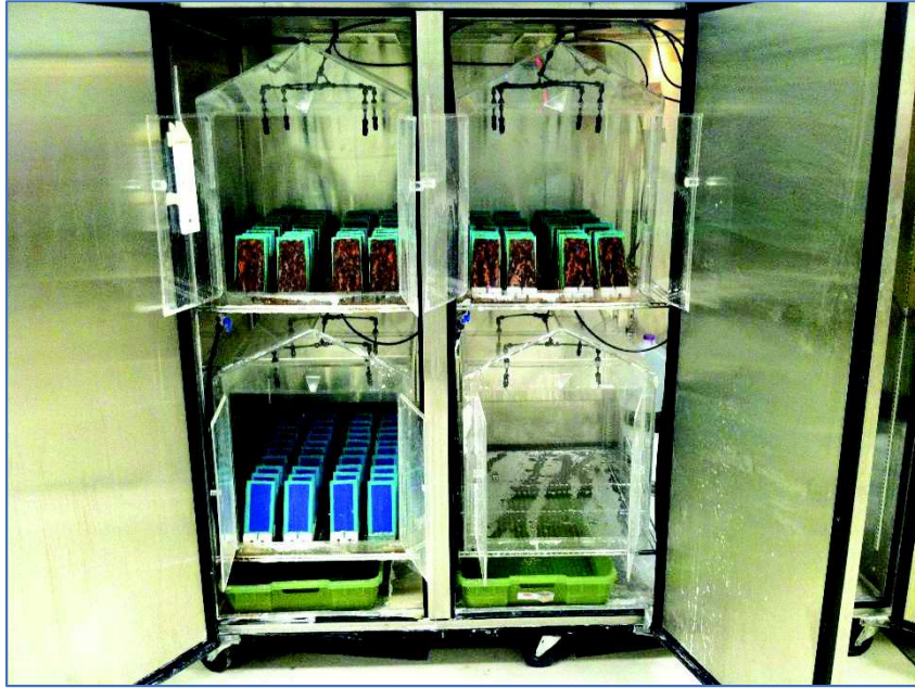
Figure 5.11: Weather chamber with steel coupons under ACT regime.
