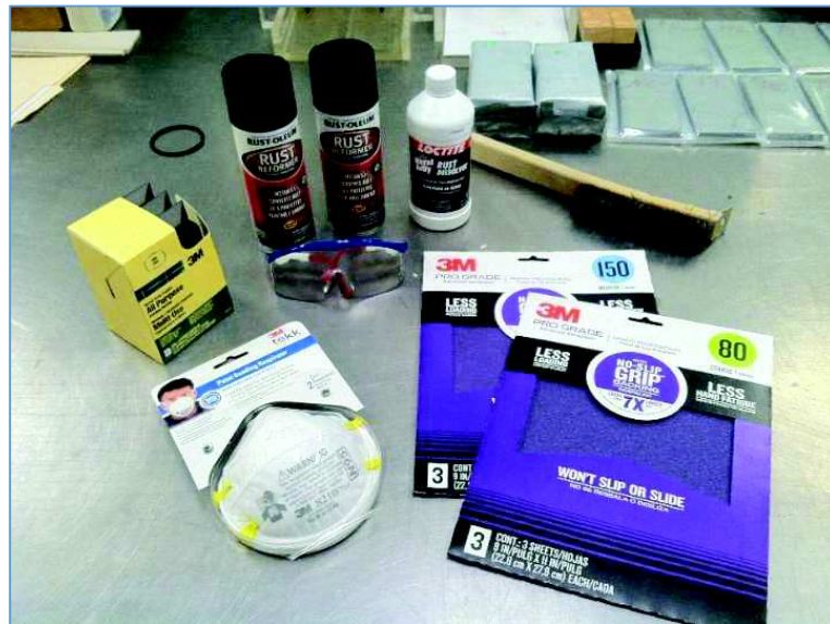
Figure 5.31: Tools and products used to eliminate the rust and protect the scribe.
