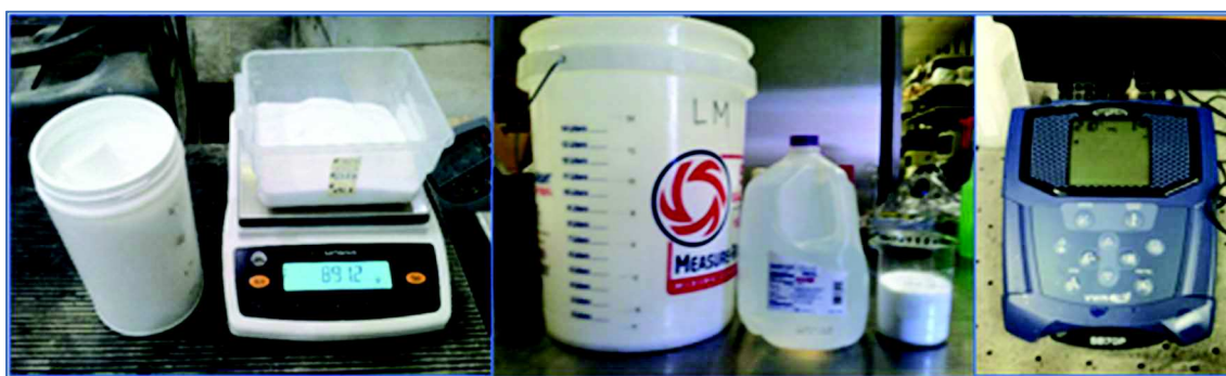
Figure 5.8: Components for salt solution preparation: Sodium chloride and scale (left), distilled water and graduated plastic bucket (center), and pH-meter (right)
