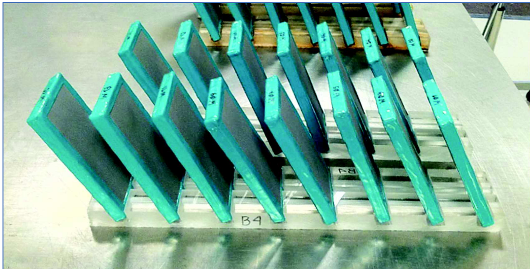
Figure 5.2: Steel coupons supported by PVC racks.
