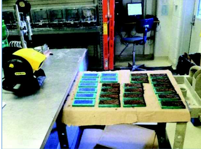
Figure 5.13: Drying wet coupons after washing
