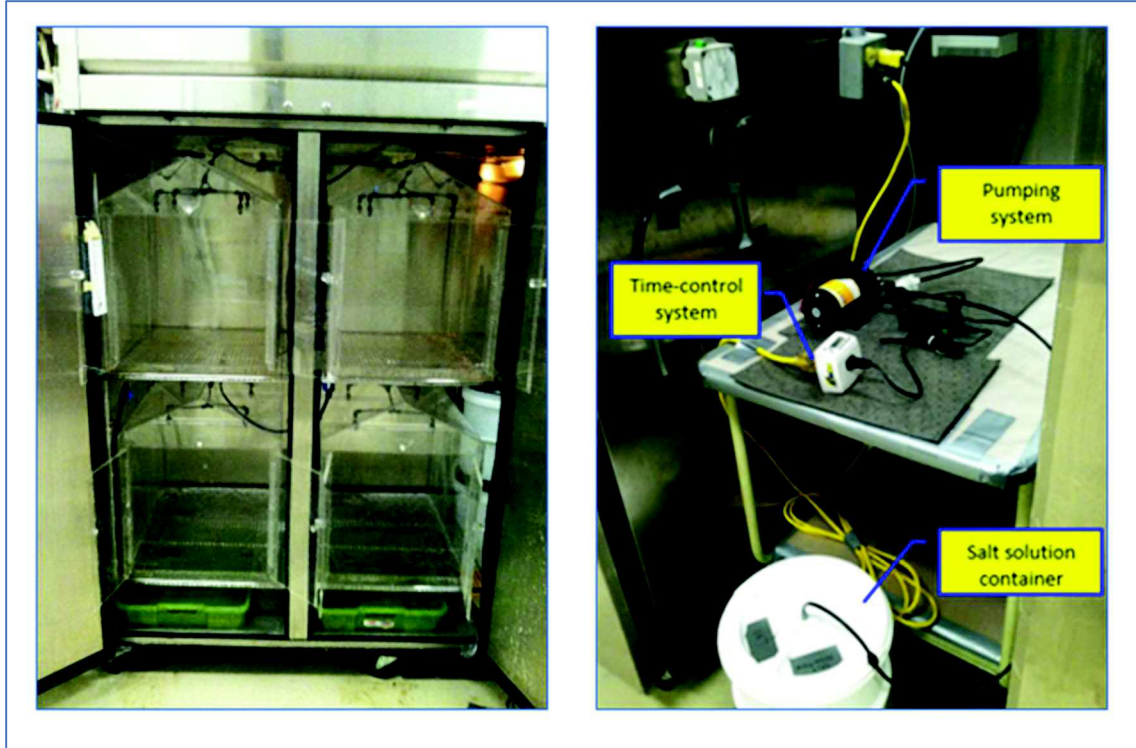
Figure 5.4: Interior view of weather chamber with acrylic boxes (left). Misting system installed (right)
