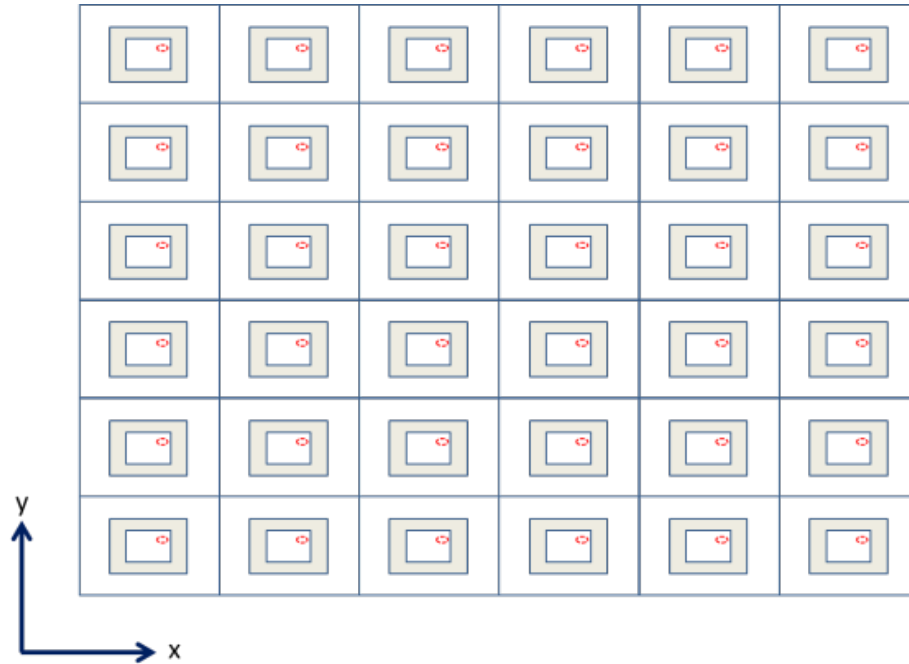
Fig. 7.15. Planar view of 6 by 6 patch antenna array.
