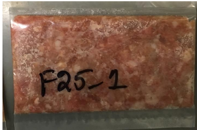
Figure 3.1 A pouch (7.6 x 12.7 cm) containing 5-g inoculated ground beef used for thermal resistance study.
