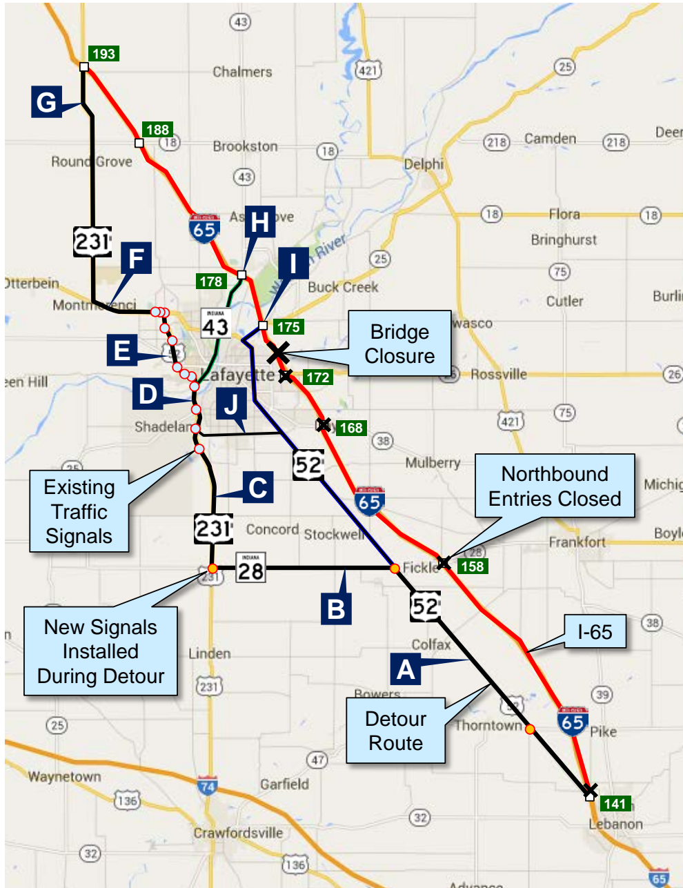
Figure 2.24 Map of the I-65 detour. The black line shows the official detour, while the blue and green lines show alternative routes. Letters A–I indicate where Bluetooth monitoring stations were located
