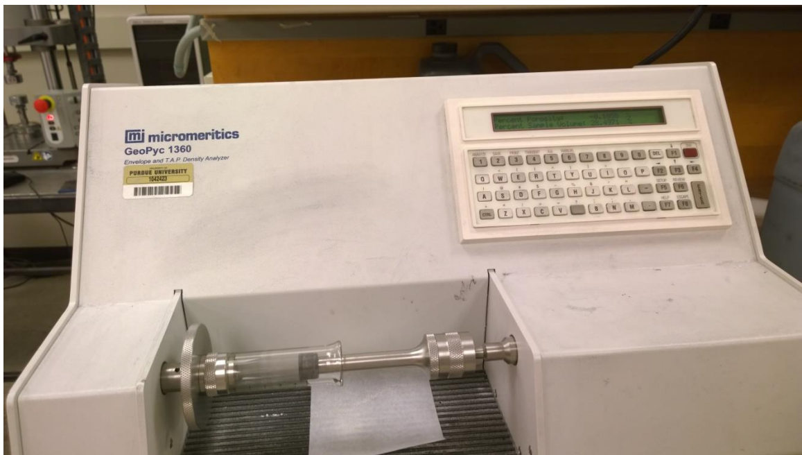
Figure 5-3 GeoPyc 1360 machine used to measure envelope density. The chamber is filled with a grain sample and DryFlo
