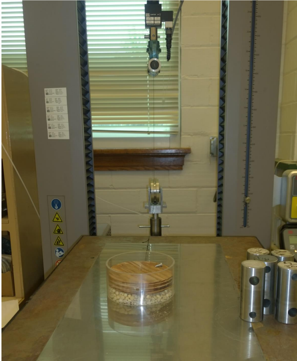
Figure 5-2 Experimental setup to measure coefficients of friction.
