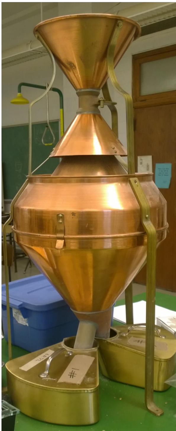
Figure 5-1 Boerner divider (Seedburo Quality, Chicago, IL) used to get a representative sample from the grain mass.
