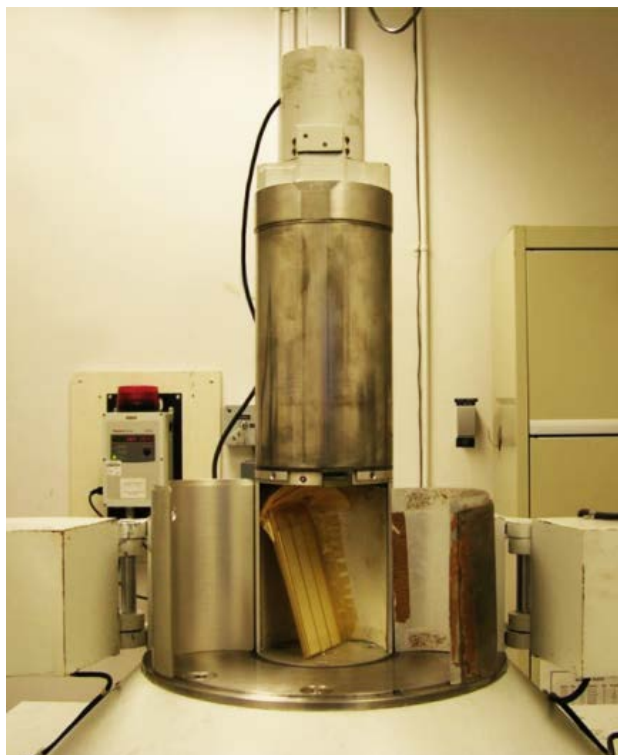
Figure 5.2. Photograph of test samples in the gamma cell.
