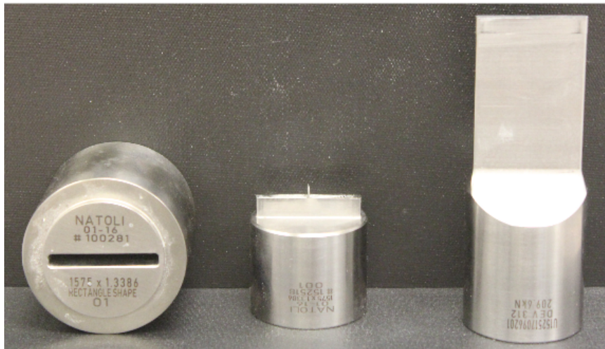
Figure 5.3. Tooling used to make compacts with v-notch for SENB fracture testing.
