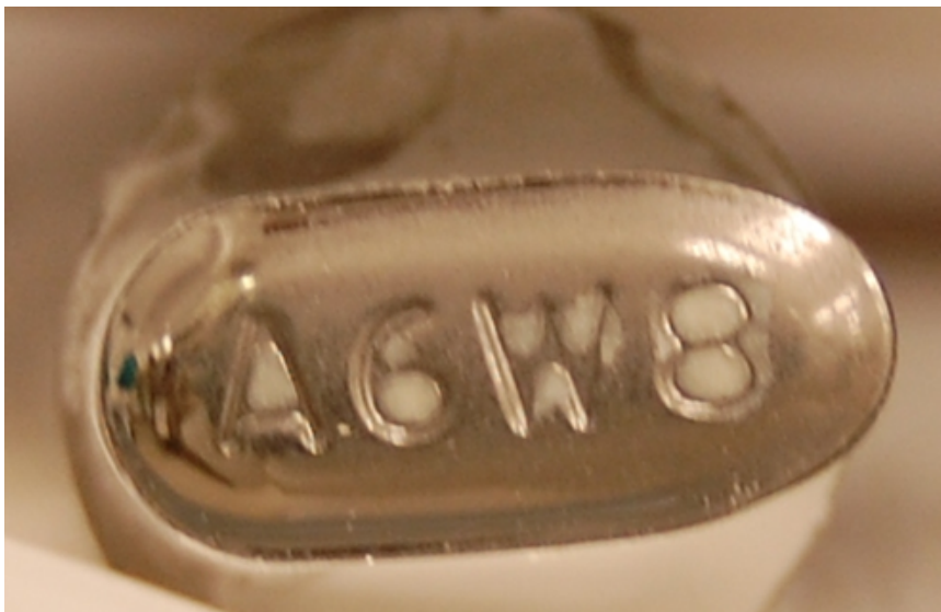
Figure 2.1. An embossed punch with the letters ‘A6W8’ commonly used as a qualitative assessment tool to evaluate the propensity of a formulation to pick and stick in the pharmaceutical industry.
