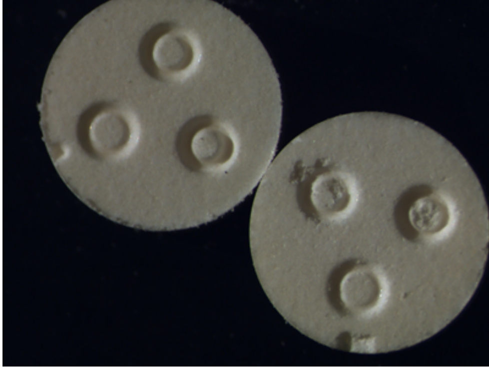
Figure 7.1. Debossed tablets produced for the experimental validation of the FEM simulation. Picking was observed in some of the tablets produced experimentally.
