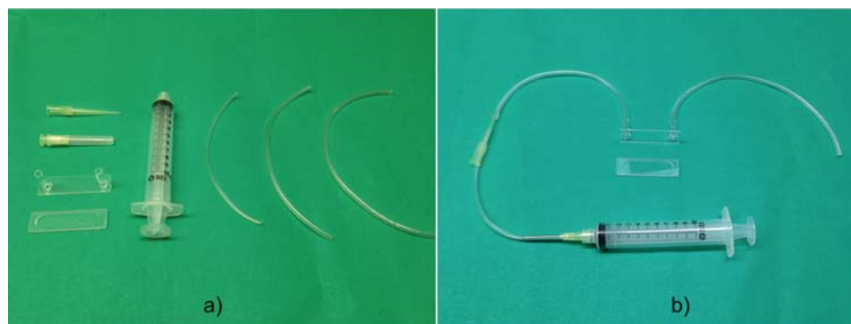
Figure 2.1. Flow cell and drug injection components. a) Drug injection components were a syringe (3-10 mL volume, depending on need), a needle (20 gauge), a pipet tip, ~3 in. of 1/32 in. inner diameter flexible tubing, and two ~3 in. pieces of 1/16 in. flexible tubing. b) Components were assembled as shown, the cut sample was placed inside the flow cell, and the device was clamped to the target stage of the DLS system.
