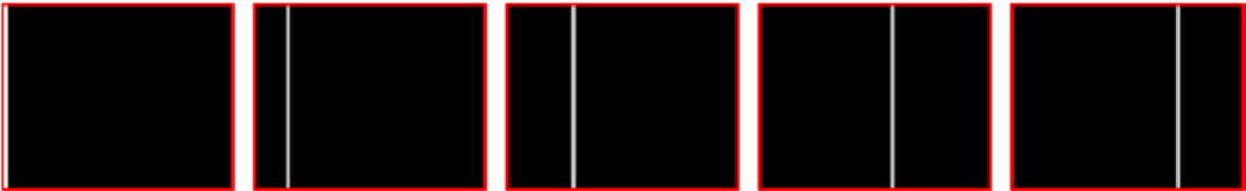
Figure 1.15: 10 mirror notches set to “1” at 0,100,200,300,400 position. The region in the white show DMD mirrors set to +12^\circ and the region in black are -12^\circ
