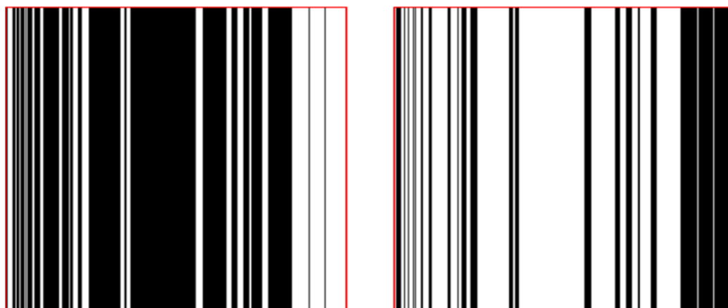
Figure 2.12: The figure shows one pair of OB-CD2 filters for acetone and benzene. Notice that they are complementary to each other and only one of these is needed to be applied to the DMD to make count measurements on both the detectors.
