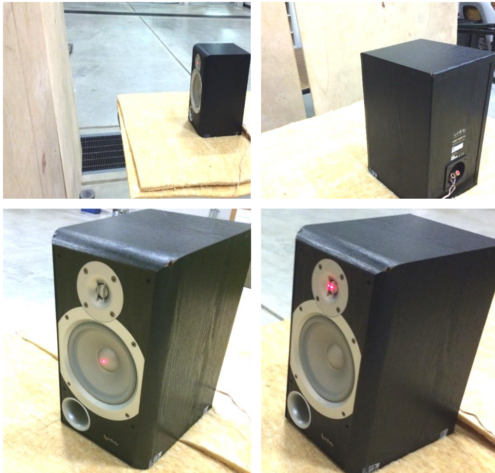
Figure 4.26. Setup of the laser vibrometer measurement of the diaphragm and the tweeter's velocity of the loudspeaker.
