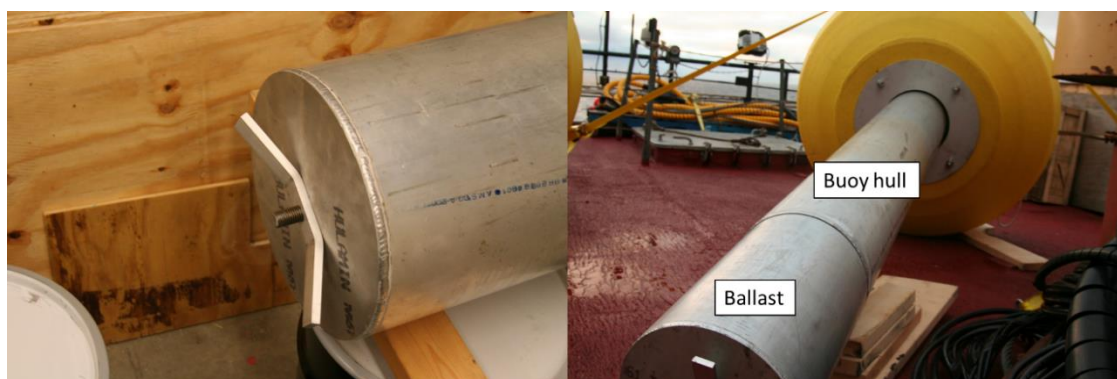
Figure 2.5 Counter-weight is an aluminum container filled with lead shot, acting as a ballast. Left- ballast is connecting to the bottom of the O-Buoy hull with threaded rod and secured into place with the winged bar. Right – Photograph of the ballast attached to the bottom of the O-Buoy hull.
