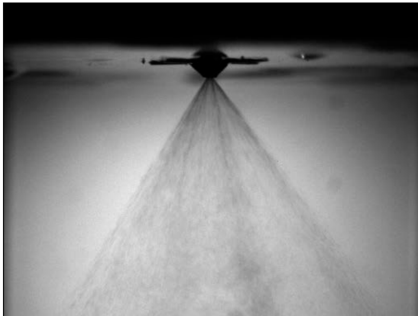
Figure 4.17 High Speed image of spray without co-flow of air. Flow number of the pressure swirl atomizer was 0.072 \text{ mm}^2
