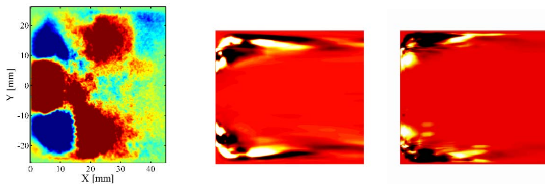
Figure 5.9: DMD spatial mode for T_{air} : 800 K and \phi : 0.6 at f : 1005 Hz from OH-PLIF signal (left) and at f : 1150 Hz from 2-step chemistry simulations (right)
