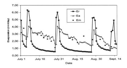
**Fig.1.** Comparison of evaporation rates estimated by Ritchie (Er) and Aydin (Ea) models, and measured evaporation (Em).
