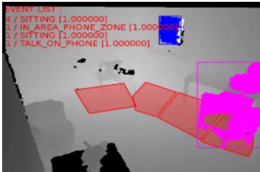
Figure 2. Visual event recognition. Event models may be defined by the spatio-temporal relations between semantic regions of the scene (e.g., table, medical cabinet, landline telephone - red polygons) and dynamics of the monitored person, like silhouette's shape (in purple) and spatial relations (e.g., closeness to the telephone table).
