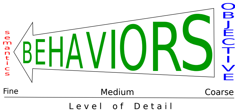
Figure 2.5: Conceptual view of how the performance of a program can be analyzed. At one extreme we have objective-based analysis, a coarse view of performance. Semantics-based analysis lies at another extreme, where a high level of detail is sought. Finally, behavior analysis provides a variable scale based on how the problem context is considered.
