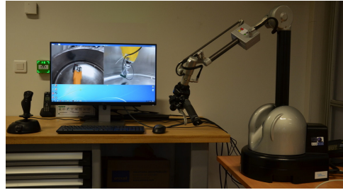
Fig. 6. Picture of the control station on CEA Tech's TROPIC platform. Joystick on the left. Camera views in the middle. Master arm Haption Virtuose 6D on the right.
