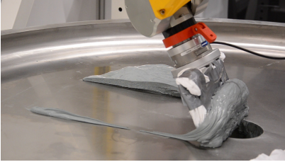
Fig. 8. Successful robotic scrubbing experiment.
