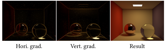
Fig. 11. Our implementation of gradient-domain path tracing at 16 samples per pixel, implemented through the conditional probability density of the shift map. The intensity of the gradients are adjusted to have a clearer view.
