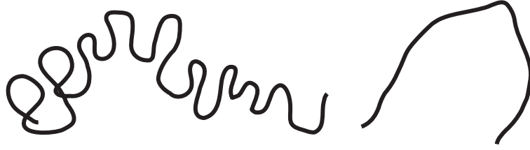
Figure 2.5: Two polymers with a different persistence length. The left polymer with a small persistence length is more flexible and changes direction over relatively short distances. The right polymer has a much larger persistence length, and therefore remains straighter.
