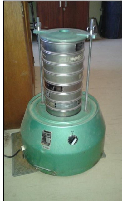
Figure 26: The Endecott test sieve shaker. Each sample is sieved for 10 minutes. Sieve mesh sizes include <math><63\mu\text{m}</math>, 63 \mu\text{m} , 125 \mu\text{m} , 250 \mu\text{m} , 500 \mu\text{m} , 1000 \mu\text{m} , 2000 \mu\text{m} , 4000 \mu\text{m} , 8000 \mu\text{m} .
