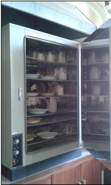
Figure 25: The Labcon forced air circulation oven. Samples are dried at 60°C for 24 hours.
