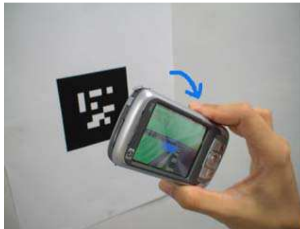
Figure 2.5: A marker based tracking system using a marker as a reference point for the camera
