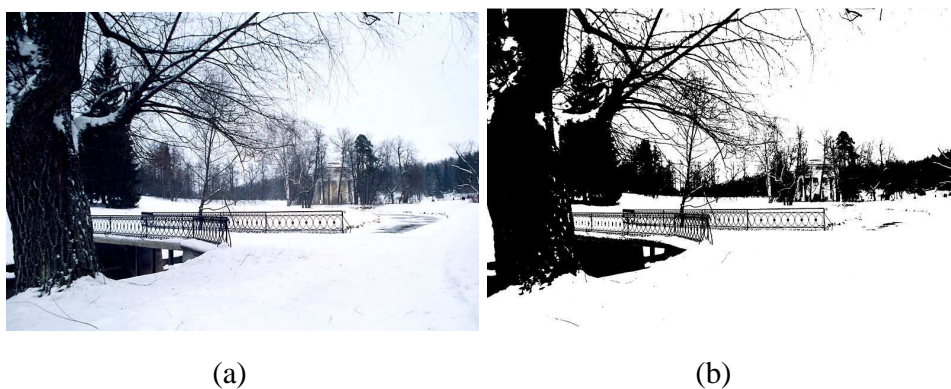
Figure 3.2: (a) shows the original image (b) shows the same figure with a threshold applied, highlighting foreground(object) and background pixels.
