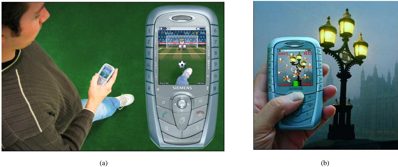
Figure. 2.7. (a) AR-soccer (Kick Real) is operated with the user’s foot as in the real game of soccer. Speed and direction are calculated when the user moves their foot to kick the virtual ball. (b): Mozzies game on the Siemens SX1 smart phone The user must move the phone and point the crosshair at the ‘Mozzies’ clicking on them to shoot them.
