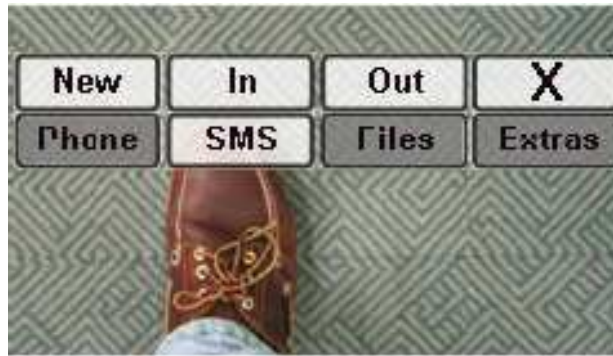
Figure. 2.6. Kick-up-menus are operated with the mobile devices camera and the users foot acting as a pointer.
