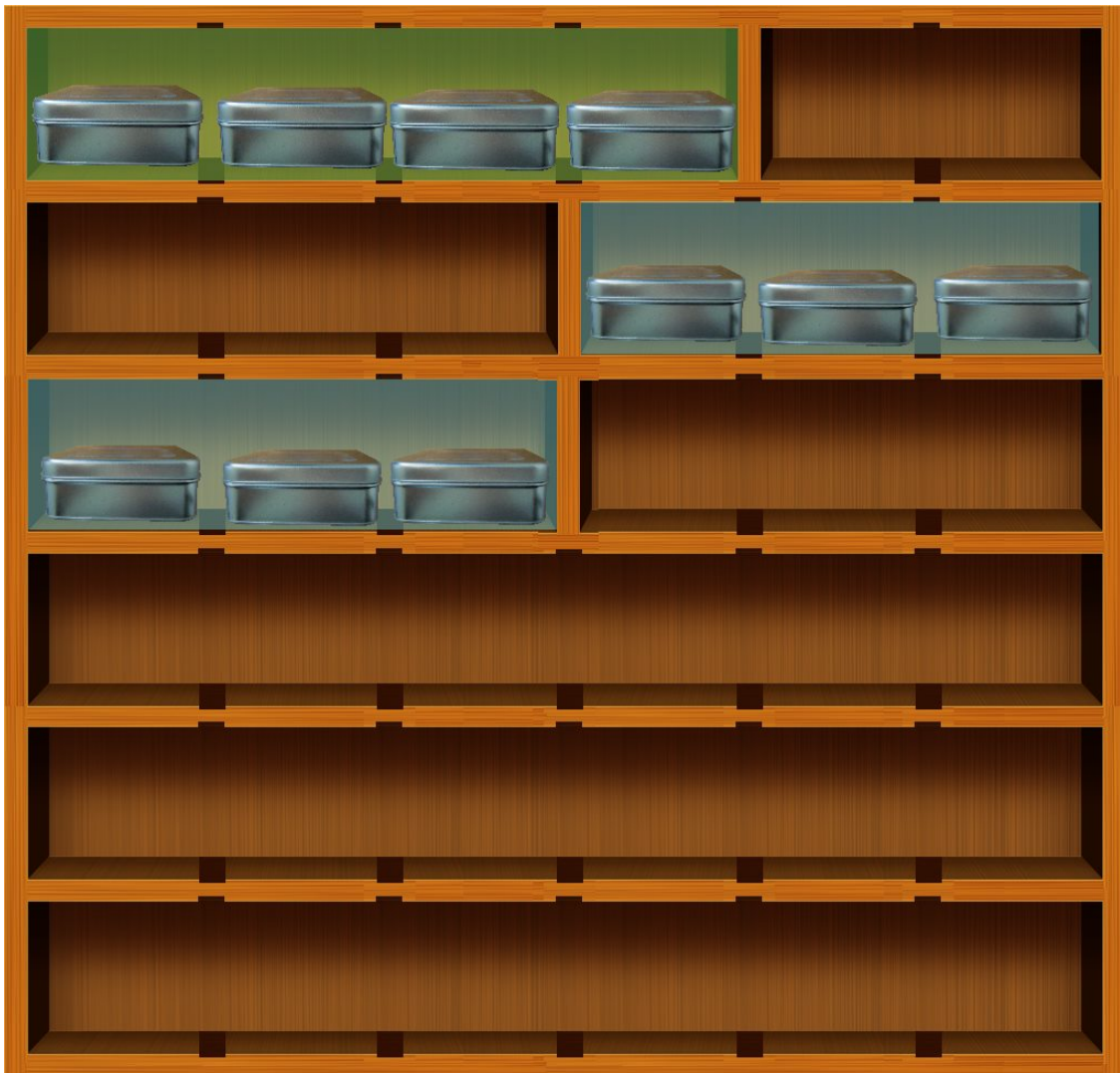
Figure 4.10: The heap bookshelf with two objects in it. If they were array objects they would be of length 4 and 6 respectively. This heap can only contain 36 simple values, and thus demonstrates how a compressed representation would be desirable.
