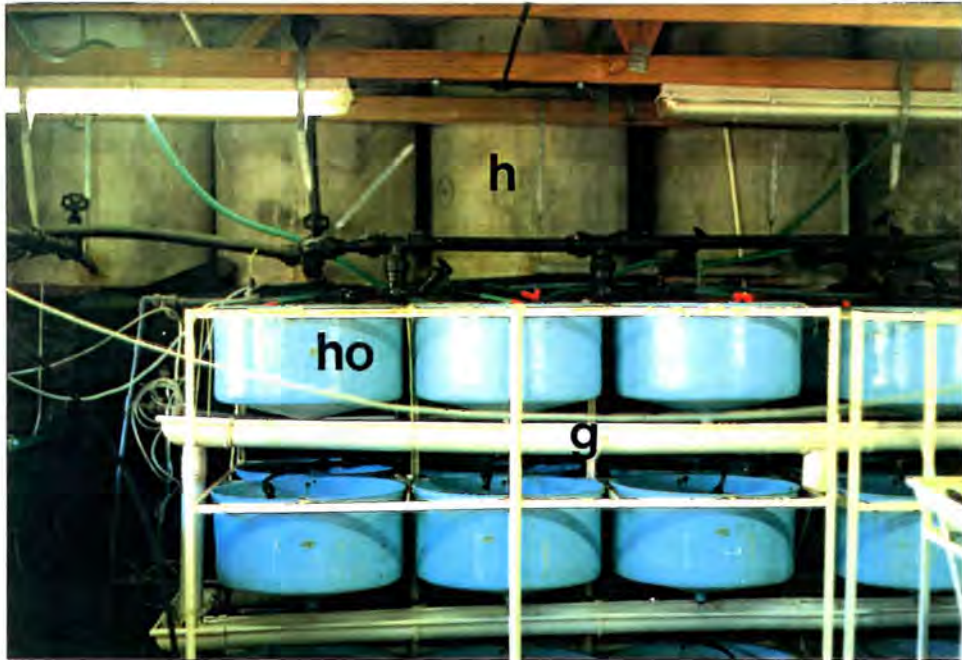
Figure 8.1 Experimental recirculating system for the housing of juvenile rainbow trout. ho = holding tank; h = header tank; g = gutter to biological filter. The biological filter is housed in a separate outdoor unit, and is not shown in the figure.
