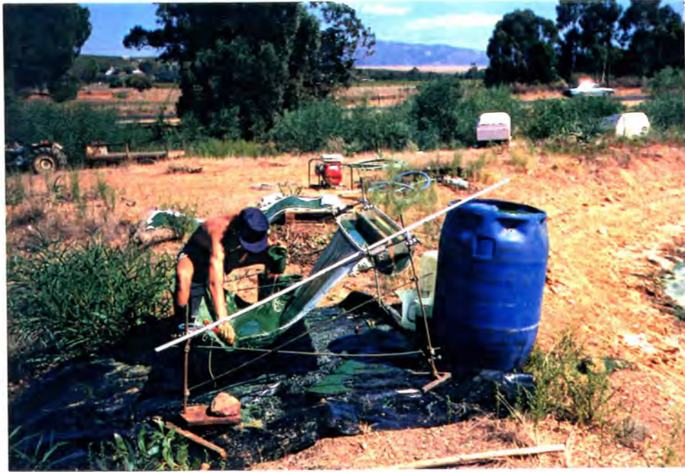
Figure 4.2 On-site operation of the screen harvester in a small-scale harvest of Spirulina biomass from tannery effluent.
