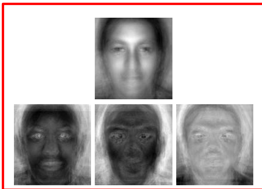
Figure 2e: A face space with a mean image (above) and three eigenfaces (below)
