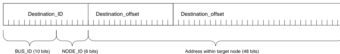
Figure 13: Destination addressing within asynchronous packet format
