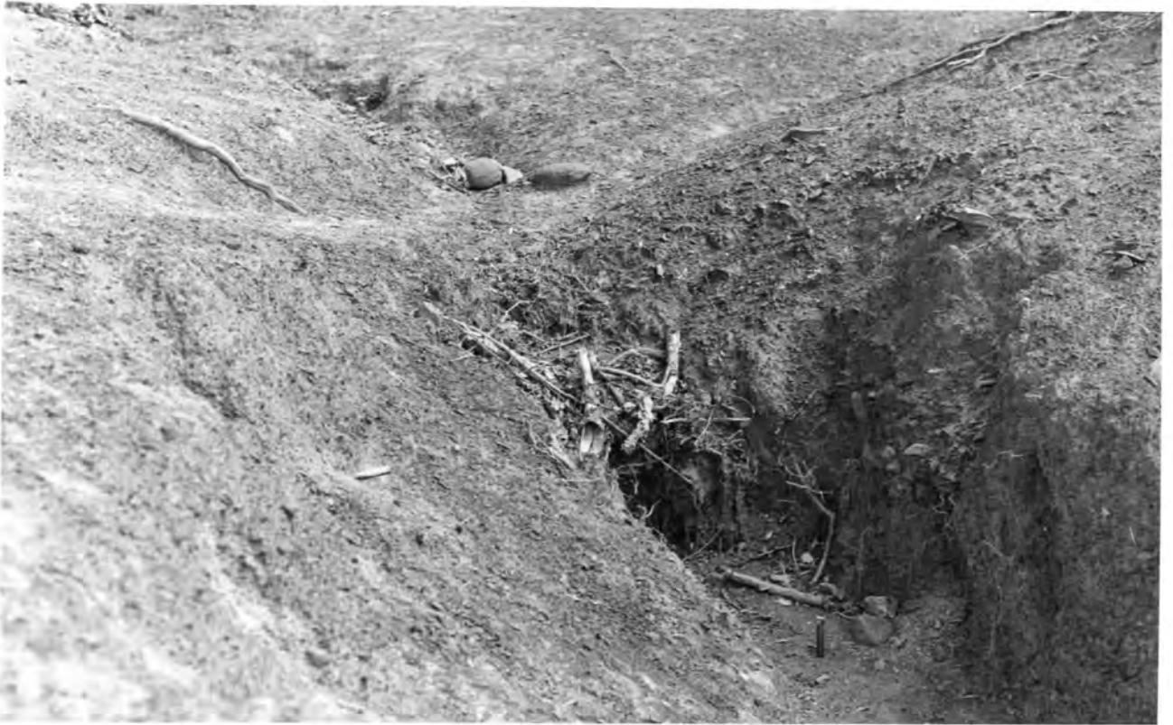
Plate 7.2a. An erosion pin in a minor rill at the tributary gully at site 5.
