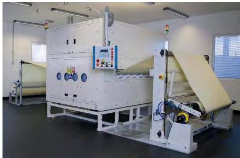
Fig.3.5 Large scale production of a nanofiber sheet by nozzle-less electrospinning line (Nanospider™) [154].
