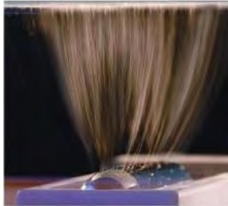
Fig.3.4 Free liquid surface electrospinning from a rotating electrode [154].
