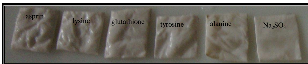
Figure 5.20: 11-mercaptoundecanoic acid stabilised copper-gold alloy nanoparticles based test strip after exposure to aspirin, lysine, glutathione, tyrosine, alanine and sodium sulphite at pH 7
