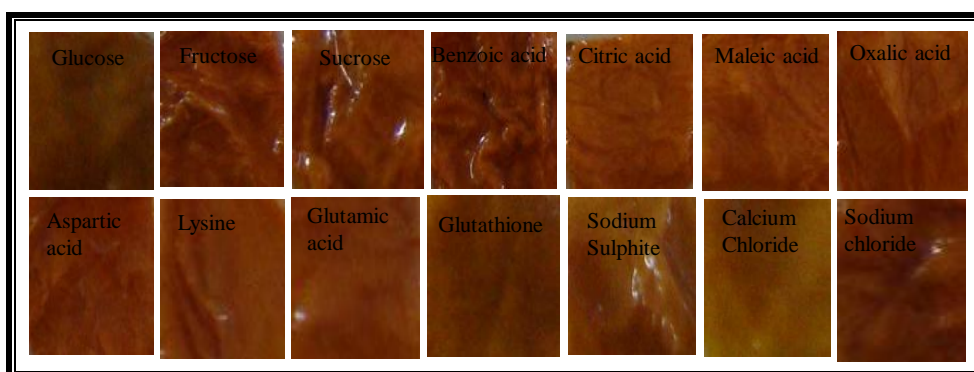
Figure 5.78: Colorimetric response of Fe(III) - 2-(2'-pyridyl)-imidazole functionalised poly(vinylbenzyl chloride) test strip in glucose, fructose, sucrose, benzoic acid, citric acid, maleic acid, oxalic acid, aspartic acid, lysine, glutamic acid, glutathione, sodium sulphite, calcium chloride, sodium chloride at pH 7
