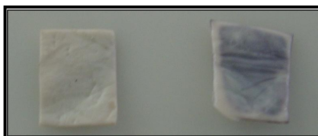
Figure 5.27: 11-mercaptoundecanoic acid stabilised copper-gold alloy nanoparticles based test strip in serum before and after fortification with 30mg L -1 of ascorbic acid
