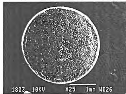
D Eudragit®RS 4% coating (surface view x 25)
