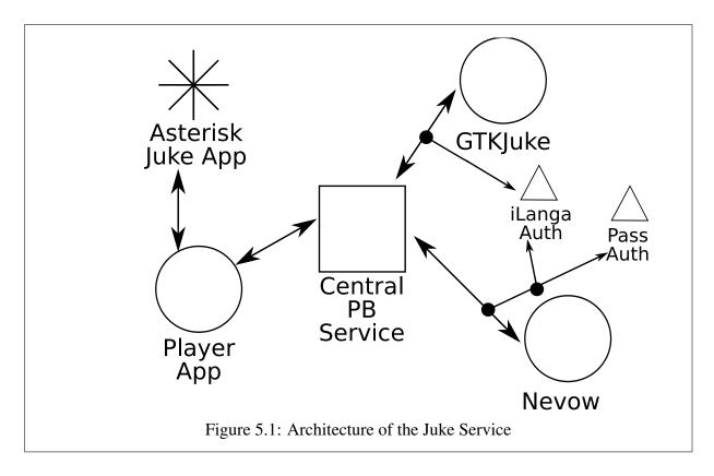
from the Nevow page. The Perspective Broker service connects the Nevow server to the Player app, which then connects the Nevow page to it. Thus, the Nevow page uses the "Pass Through" authentication method to indirectly authenticate itself to the Perspective Broker service, and gain access to the Player application. This "Indirect Authentication" method is described below in 5.7.
