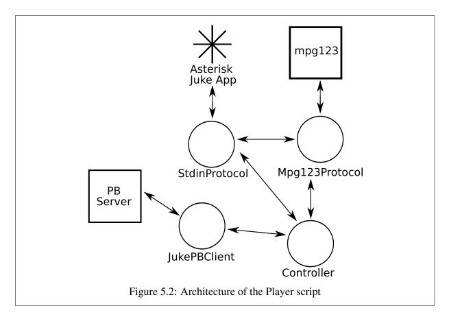
we want to use Perspective Broker, this script will need to be re-implemented in Python/Twisted. This is not actually too much of an issue, since Twisted's built-in asynchronicity will remove the necessity for the non-blocking reads that took up much of the Perl script.
