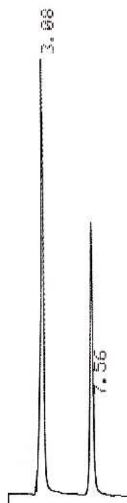
Figure 3.8. Typical HPLC chromatogram of CPT (50 \mu\text{g/ml} ) in the presence of the I.S. CYC (20 \mu\text{g/ml} )
