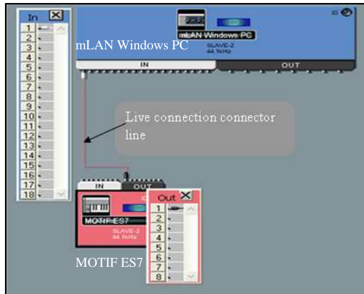
Figure 3.14: mLAN Graphic Patchbay – Successful Connection [Yamaha Corporation, 2004b]
