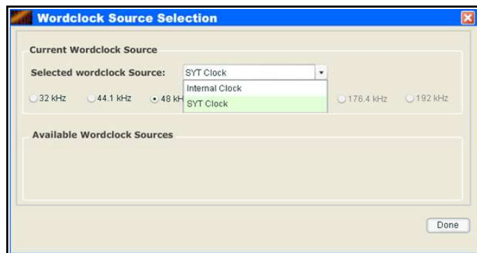
Figure 5.17: Setting the Word Clock Source and Sample Rate
