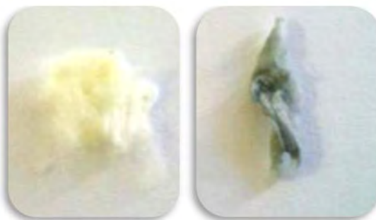
Figure 5.22 Digital images of p(ST-co-VPIM) (left) and p(ST-co-VPIM)-VO fibers (right) showing the significant colour change upon functionalization
