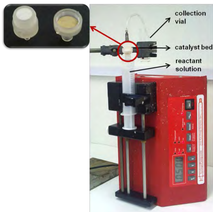
Figure 5.5 Continuous flow set-up, when using \text{PBI}_7\text{-VO} fibers. The insert shows an expanded view of the catalyst bed
