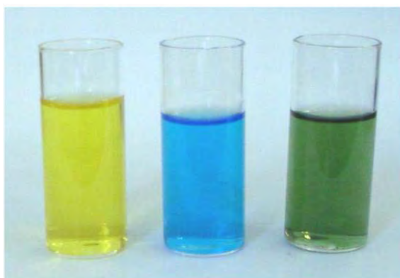
Figure 1.11 The colour of vanadium in biologically relevant oxidation states. From left to right, V^{5+} , V^{4+} , V^{3+}
