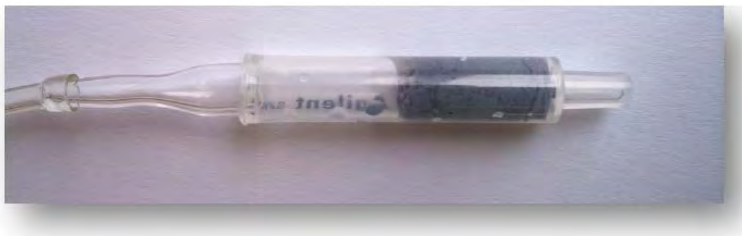
Figure 5.38 The modified column used in the continuous flow reactions, containing the p(ST-co-VPIM)-VO fibers (0.1 g)
