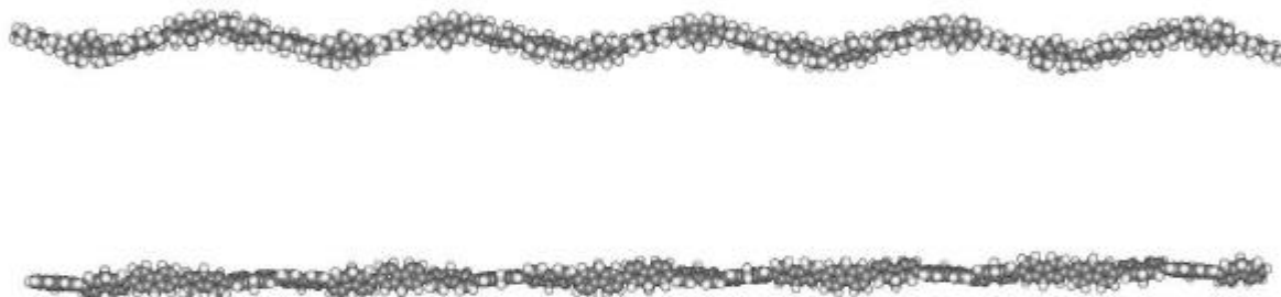
Figure 5.8. Molecular Modeling of oligo(25)-fluorene with 5/q helix. (Up): q = 1 ; (Down): q = 2 . Structures are based on RHF/6-31G calculations of bi- and terfluorene. Ethylhexyl side chains were replaced by hydrogen.
