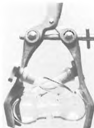
PLATE 1: In vitro cells in laboratory clamp for steady-state permeation experiments.
