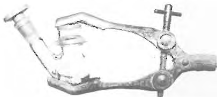
PLATE 2: In vitro cells in laboratory clamp for in vivo -mimic permeation experiments.
