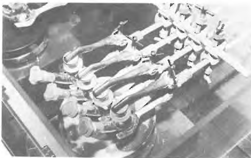
PLATE 3: Arrangement of four in vivo -mimic cells in water bath above magnetic stirrer.
